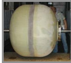
Liner Pressure Test
