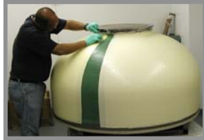
Tank Liner Lamination
