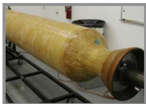
CTN Insulator with AAE Aerospace's Ablative Nozzle
