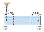
Carefully heat the Plexiglas<sup>™</sup> along the dotted line drawn 4 cm from each end. Heat one end at a time, bending the Plexiglas<sup>™</sup> to 90°.
