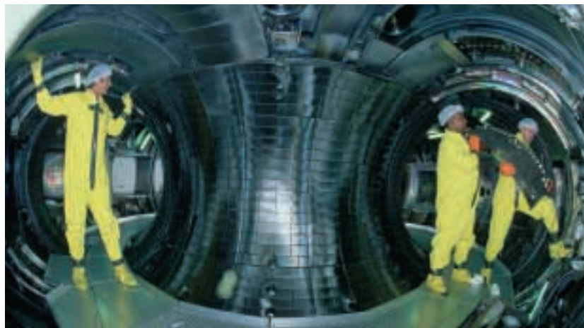
Figure 21.7 These workers are inspecting the inside of the experimental Tokamak fusion reactor at Princeton University.
