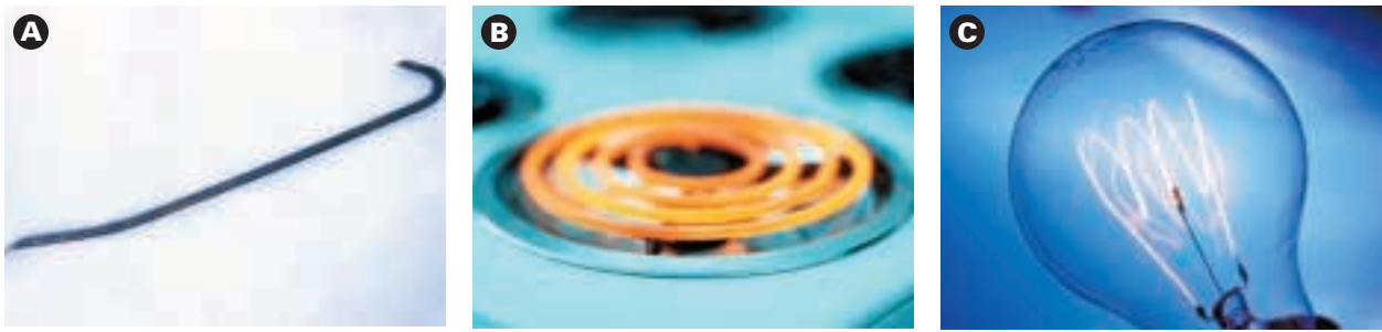
Figure 18.3 (A) While an object such as a crowbar emits no visible radiation at room temperature, it is actually emitting infrared radiation. (B) When a stove coil reaches 600 K, it emits mostly invisible, infrared radiation. The radiation appears to be red, because it emits a little visible radiation in the red end of the spectrum. (C) At 2000 K, a light bulb filament looks white, because it emits all frequencies in the visible range.
