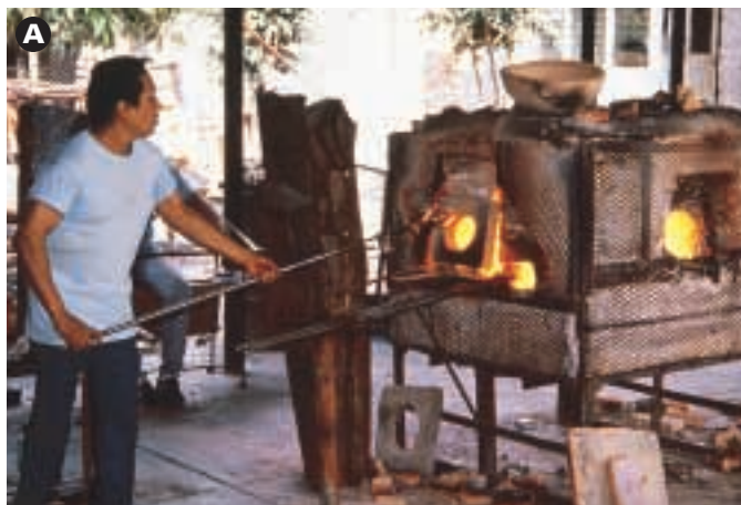
Figure 18.1 (A) When the temperature of a kiln surpasses 1000 K, the radiation is independent of the nature of the material in the kiln and depends only on the temperature. (B) A tiny hole in a very hot cavity “samples” the radiation that is being emitted and absorbed by the walls inside.
