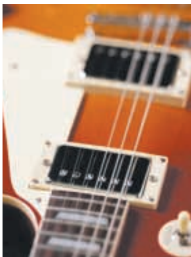
Figure 16.30 Electric guitar pickups rely on Lenz's law.
