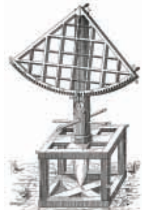
Figure 12.2 Brahe’s observatory in Hveen, Denmark, contained gigantic instruments that, without magnification, were precise to 1/30 of a degree.
