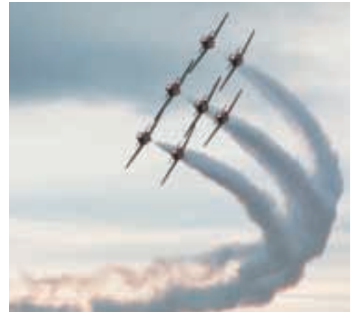
Figure 11.10 When an airplane follows a curved path, it must tilt or bank to generate a centripetal force.
