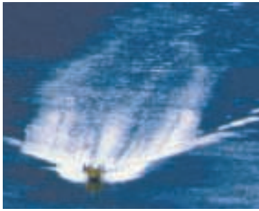
Figure 9.20 The large bow wave is the result of the boat moving faster than the speed of the waves in water.
