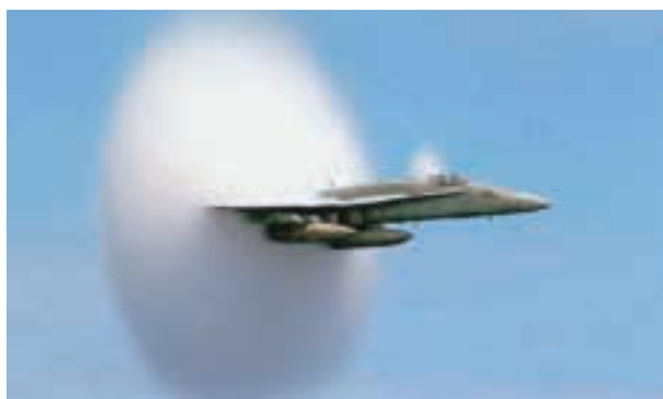
Figure 9.18 The shock wave as a jet breaks the sound barrier is visible because the increased pressure causes water vapour to condense.
