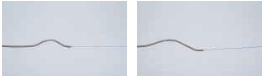
Figure 8.12 When a wave pulse is reflected from a free end, the reflected pulse is on the same side as the original pulse.
