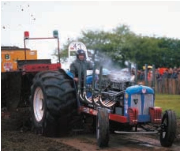
Figure 5.6 In a tractor pull, vehicles develop up to 9000 horsepower to accelerate a sled, until they can no longer overcome the constantly increasing frictional forces. Dragsters, on the other hand, accelerate right up to the finish line.
