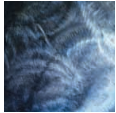
Figure 4.7 Highly polished steel that feels very smooth still has bumps and valleys that will collide with other surface imperfections when rubbed together.
