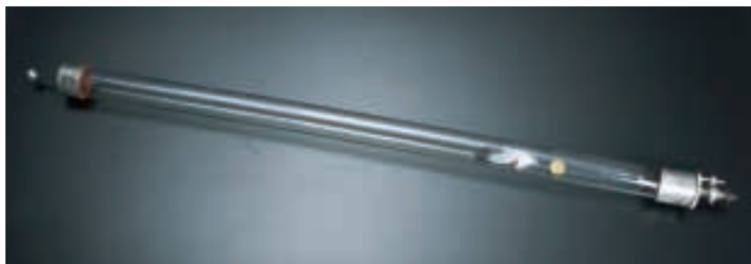
Figure 4.5 Acceleration due to gravity does not depend on mass, as demonstrated by the example of the feather and the coin in a vacuum tube.
