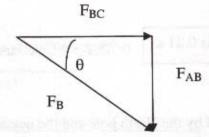
$$\begin{split} F_B^{\ 2} &= F_{BC}^{\ 2} + F_{AB}^{\ 2} \\ F_B^{\ 2} &= (8.07 \times 10^3 \, \text{N})^2 + (1.42 \times 10^4 \, \text{N})^2 \\ F_B &= 1.63 \times 10^4 \, \, \text{N} \\ \end{split} \qquad \begin{aligned} \tan \theta &= \frac{F_{AB}}{F_{BC}} \\ \tan \theta &= \frac{1.42 \times 10^4 \, \text{N}}{8.07 \times 10^3 \, \text{N}} \\ \tan^{-1}(1.76) &= \theta \\ \theta &= 60.4^\circ \end{aligned}$$
