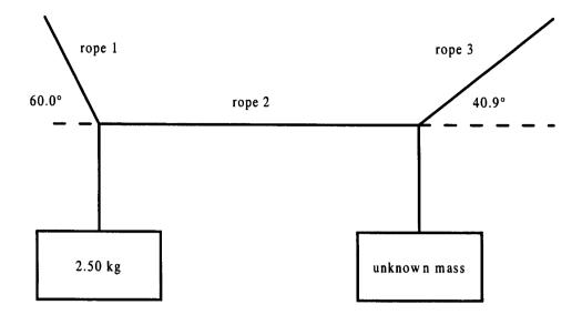
Two signs are suspended in equilibrium using three ropes of negligible mass as shown above. The sign on the left has a mass of 2.50 kg, and the rope connecting it to the ceiling makes an angle of  $60.0^{\circ}$  with the horizontal. The rope connecting the sign on the right to the ceiling makes an angle of  $40.9^{\circ}$  with the horizontal. Determine the mass of the sign on the right.
