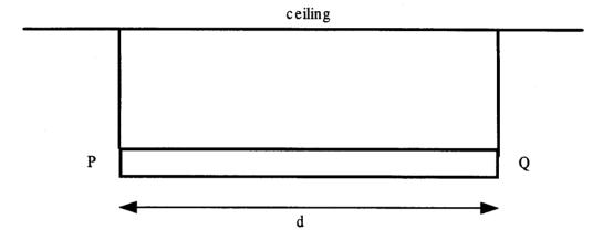
If the tension in the right hand cord is T<sub>r</sub>, what is the sum of the torques about point P?
