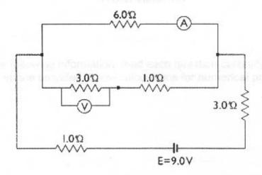
A) Calculate the equivalent resistance of the circuit. value: 3
