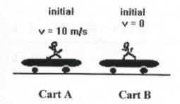
Two people of identical masses are on two identical carts, A and B. Cart A, with an initial speed of  $10\frac{m}{s}$ , collides with cart B, which is at rest. In order that this collision be perfectly elastic, what would have to be the speed of cart B, relative to the ground, after the collision?
