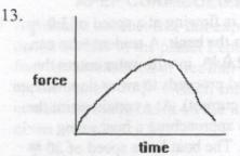
The graph shown above is the plot of a collision force of a car hitting a wall during a time interval. What physics quantity does the area under the curve give?
