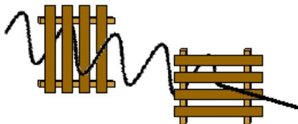
When the pickets of the second fence are horizontal, vertical vibrations which make it through the first fence will be blocked.
