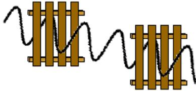
When the pickets of both fences are aligned in the vertical direction, a vertical vibration can make it through both fences.
