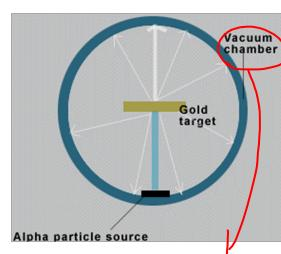
to minimize scattering of the alpha particles
